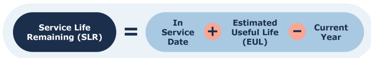
Figure 7 Service Life Remaining Calculation
