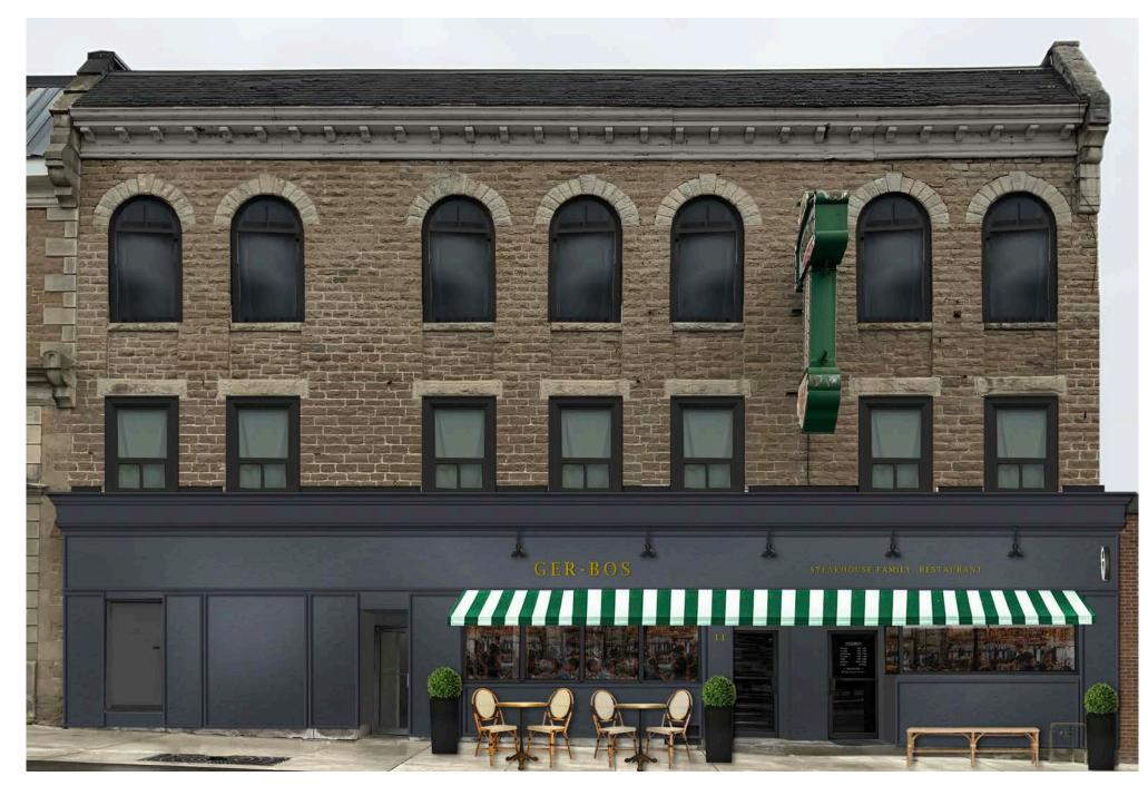
ADDITIONAL NOTES: 1) REMOVE EXISTING SHINGLED ROOF EDGE, ACRYLIC SIGNAGE. 2) INFILL EXISTING ARCHED RECESSES ABOVE WINDOWS. 3) REMOVE EXISTING MASONRY FINISH AND PREP SUBSTRATE FOR NEW METAL PANELS. 4) ADD J-BOXES FOR NEW GOOSE LAMPS.
