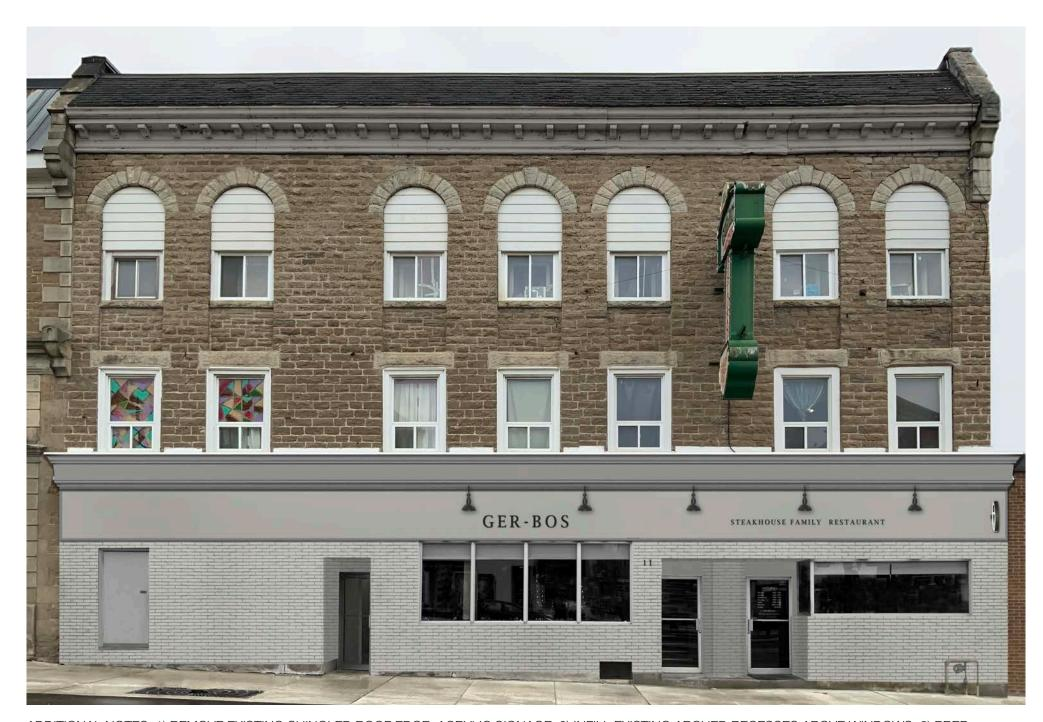
ADDITIONAL NOTES: 1) REMOVE EXISTING SHINGLED ROOF EDGE, ACRYLIC SIGNAGE. 2) INFILL EXISTING ARCHED RECESSES ABOVE WINDOWS. 3) PREP EXISTING MASONRY BASE FOR NEW PAINT FINISH. 4) ADD NEW FLAT PANEL AND CORNICE AT LOWER LEVEL. 5)) ADD J-BOXES FOR NEW GOOSE LAMPS.
