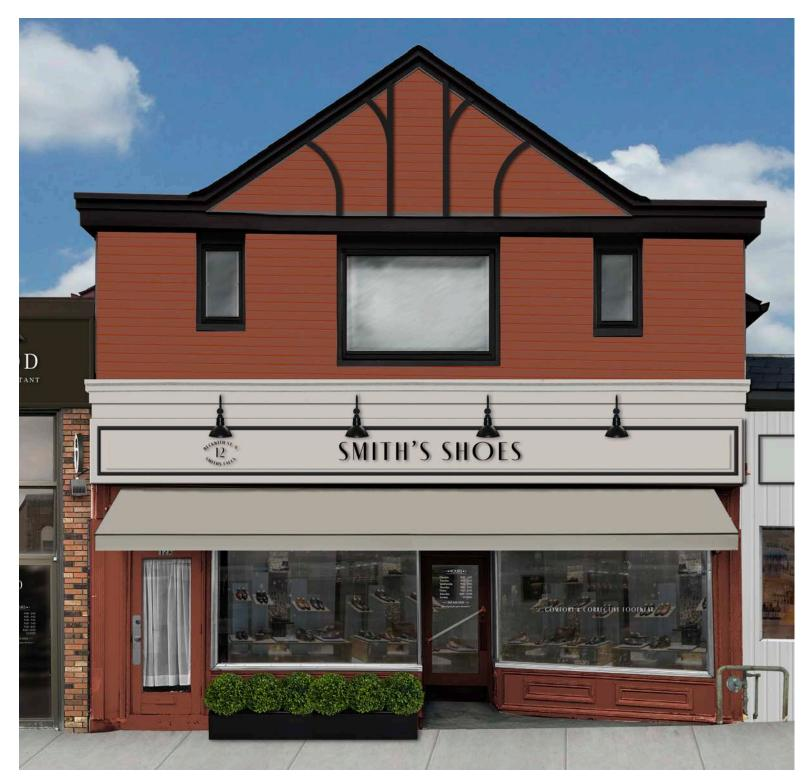
ADDITIONAL NOTES: 1) REMOVE EXISTING 3-PART WINDOWS, AWNING, AND ACRYLIC SIGNAGE. 2) INSTALL NEW PICTURE WINDOW IN EXISTING ROUGH-OPENING. 3) NEW SIGNAGE PANEL AND CORNICE DETAIL. 4) ADD J-BOXES FOR NEW GOOSE LAMPS.
